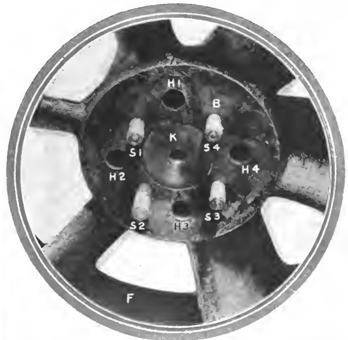
Fig. 2—Boss of the flywheel showing the studs that have been damaged through incompetent fitting
